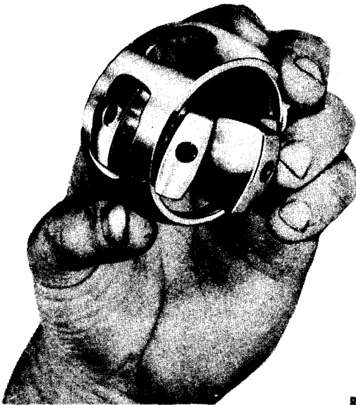
Figure 41 — Removing Inner Race From Cage (Rzeppa Joint)
