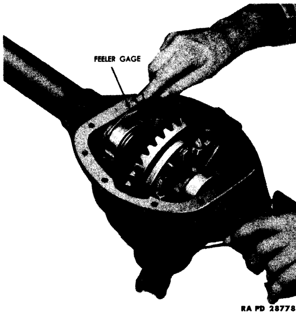
Figure 69—Checking Clearance Between Differential Case and Bearing
